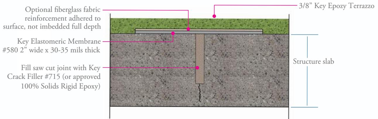
Treatment of contraction joints (sawcuts) and cracks is done in anticipation of horizontal movement.
